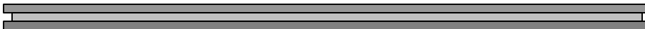
The Base Each part is about 1/2" thick. Completed thickness is about 1 1/4" to 1 1/2"
